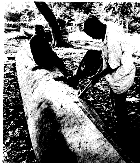
Fig. 35. Cutting a dori hull from a saba log, Tasbapauni.
